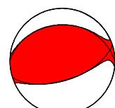
P-axis; azimuth: 169°, plunge: 15° - T-axis; azimuth: 320°, plunge: 73°
